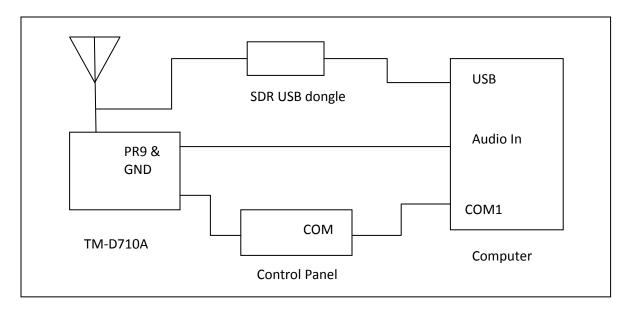
Connect the PR9 pin from the DATA connector on the transceiver to the audio input on the computer. This has wider bandwidth than the PR1 signal or the speaker output.
